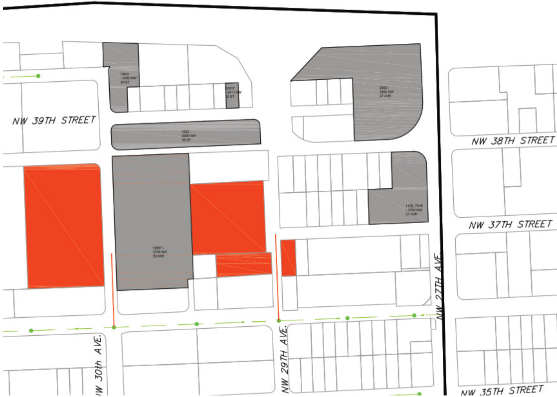
Figure 4: Proposed Gravity Sanitary Sewer with Sufficient Soil Cover (shown with red lines) [Source: HDR 7/30/2015 Draft Technical Memorandum]
